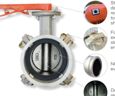
Stainless steel square shaft design minimizes rounding or releasing of disk and increases torque potential for positive shut off.
